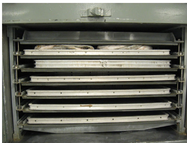
Figure 2. Two fish blocks in a contact thawer, a converted horizontal plate freezer.
