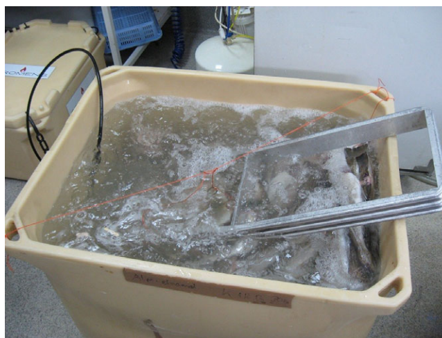
Figure 1. Fish blocks under air-assisted thawing in a 1000 L fish tub. The air bubbles were generating circulation for enhanced overall heat transfer.
